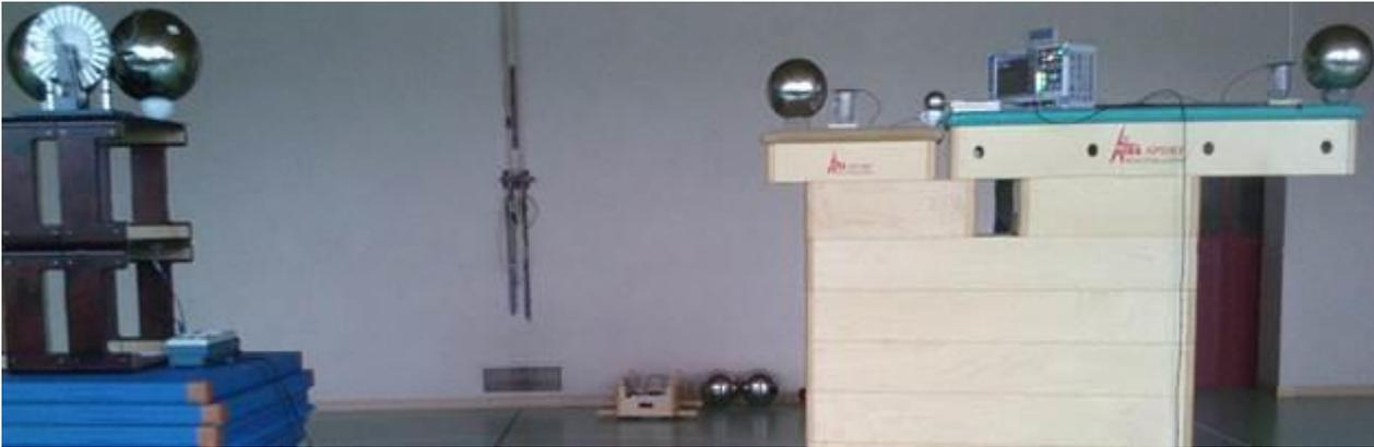
The emitter on the left consists of two metallic spheres forming a spark gap. In order to charge the dipole-spheres, a [Wimshurst influence machine](#) is used. As the spheres are used as high-voltage capacitors, the capacitor of the influence machine has been disconnected.
